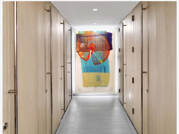
unique 3-part aluminum headrail system, the full height stalls offered maximum privacy to employees with 20mm floor and ceiling clearances.
